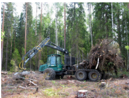
Figure 23. Forwarding of logging residues in a clear-cut operating area (Juha Laitila)
