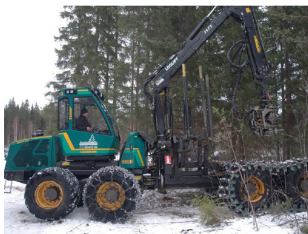
Figure 20. Forwarder based harwarder for mechanised logging of small diameter thinning wood (Moisioforest)
