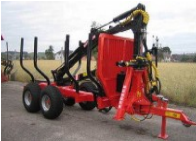
Figure 4. Tractor forest trailer and tractor with winch/skidder (LK Niederösterreich)
