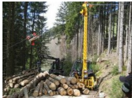
Figure 4. Tractor forest trailer and tractor with winch/skidder (LK Niederösterreich)
