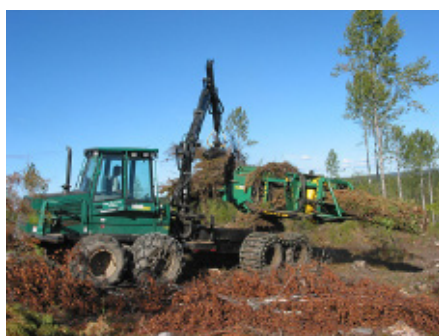
Figure 24. Forwarder-mounted logging residue bundler in a clear-cut area (Juha Laitila)
