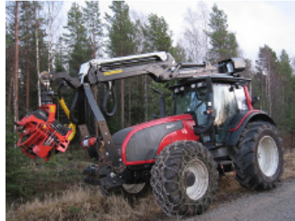
Figure 22. A forestry-equipped farm tractor (Juha Laitila)
