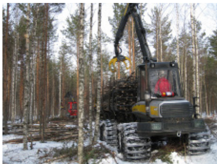
Figure 19. Traditional two-machine system for mechanised logging of small diameter thinning wood (Juha Laitila)
