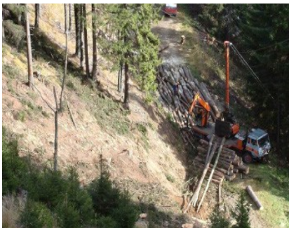
Figure 4. Tractor forest trailer and tractor with winch/skidder (LK Niederösterreich)
