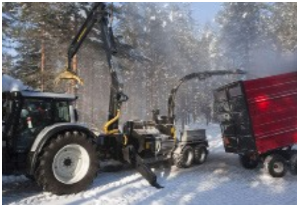
Figure 14. Farm tractor-driven chipper operating at the roadside landing (Kesla)
