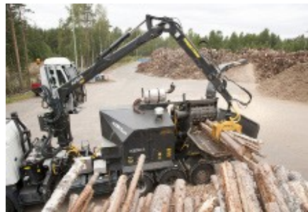
Figure 15. Heavy truck-mounted chipper comminuting large-sized roundwood at the terminal (Kesla)
