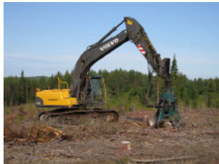
Figure 18. Harvesting of stumps at clearcut area with a single-grip stump harvester (Juha Laitila)
