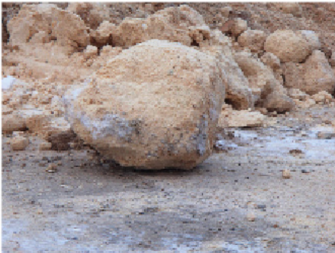
Figure 30. Large ice pieces may break conveyors and boilers (Miina Jahkonen, 2013)
