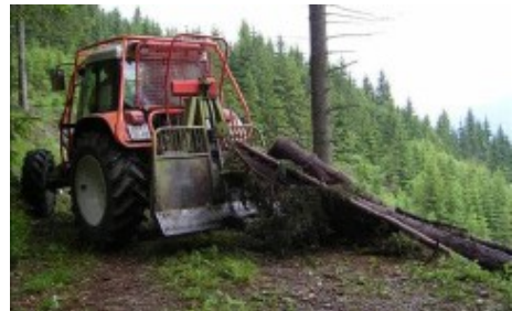
Figure 4. Tractor forest trailer and tractor with winch/skidder (LK Niederösterreich)
