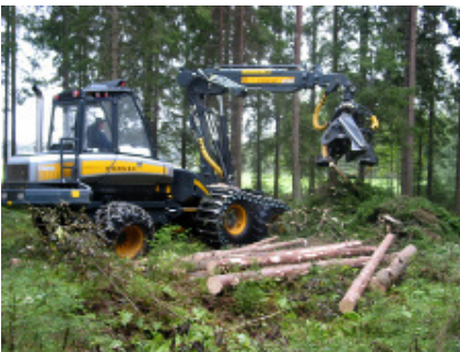
Figure 17. Integrated cutting of industrial roundwood and logging residues with a single-grip harvester (Juha Laitila)
