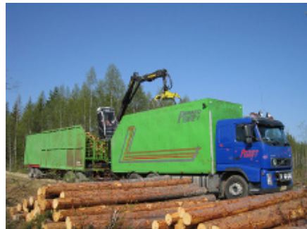
Figure 26. Biomass truck equipped with solid side panels and bottom (Juha Laitila)
