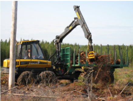
Figure 25. Forwarding of stump and root wood in a clear-cut area (Juha Laitila)
