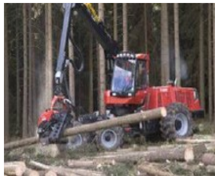
Figure 3. Felling technologies, chain saw – harvester (LK Niederösterreich)
